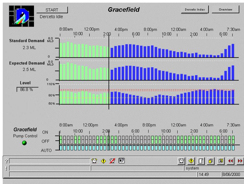
Figure 5. Operator screen for Gracefield reservoir pump schedule
