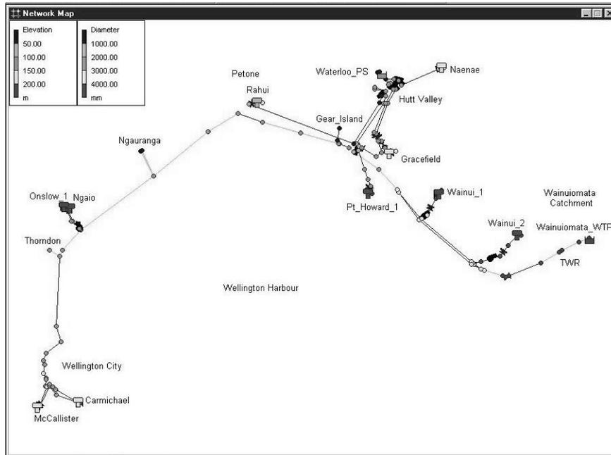
Figure 3. EPANet Model of Wainuiomata-Waterloo System
