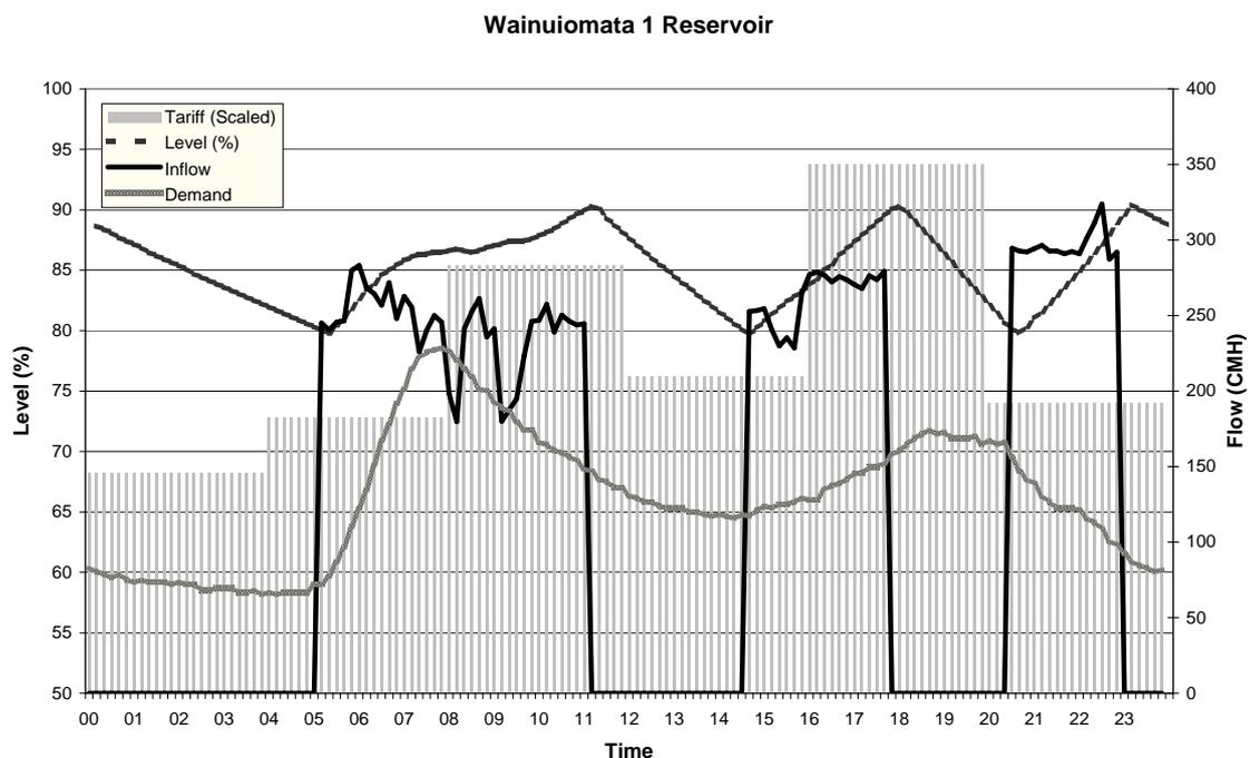
Figure 1. A Typical Reservoir under Level Control
