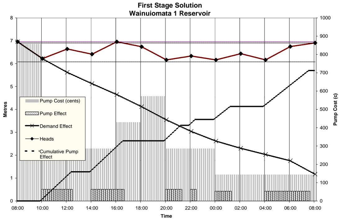
Figure 2. Sample First Stage Solution
