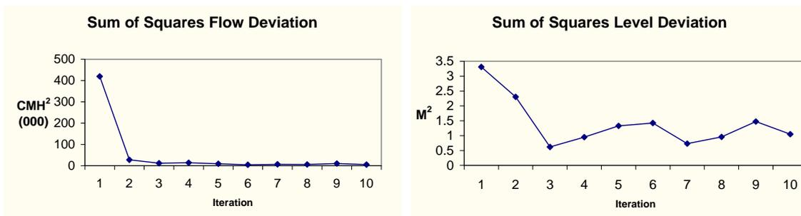
Figure 4. Head and Flow Deviation per EPANet Iteration
