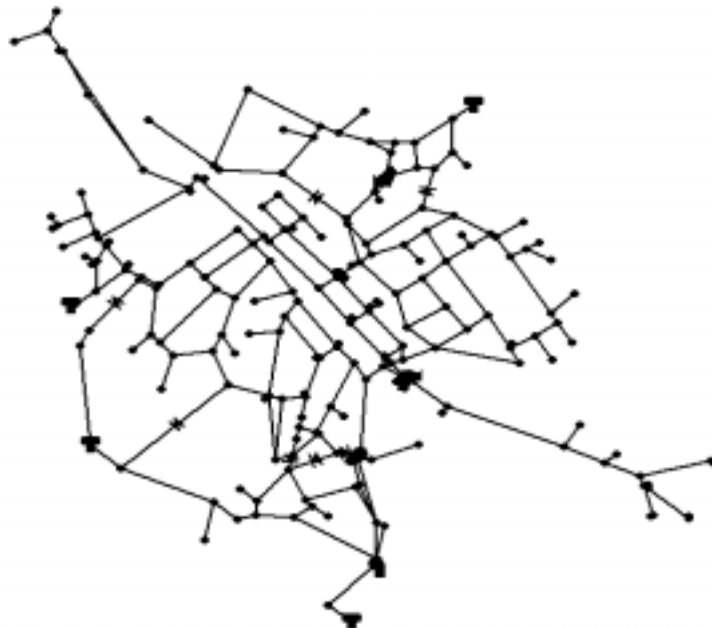
Figure 1. A Typical Water Distribution Network
