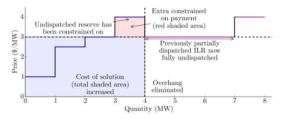
Figure 4: Example of reserve dispatch solution using constrained on payment.
