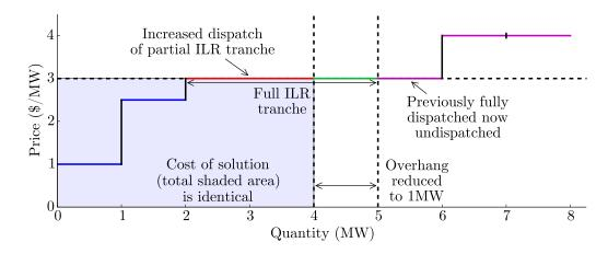
Figure 3: Example of reserve dispatch solution using intelligent selection.
