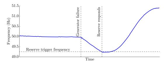
Figure 1: Example of under-frequency event with a reserve over-response.
