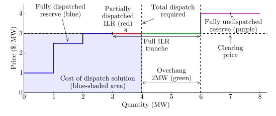
Figure 2: Example of reserve dispatch solution containing overhang.
