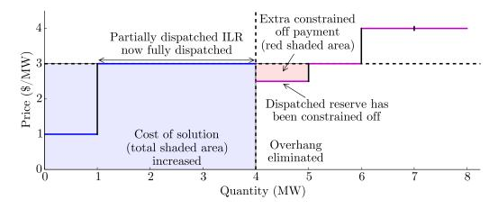
Figure 5: Example of reserve dispatch solution using constrained off payment.
