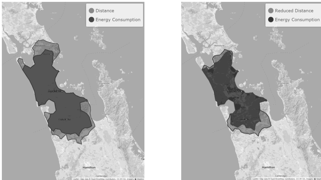
Figure 2. Nissan Leaf reachable region, comparing formulations using distance and using energy consumption
