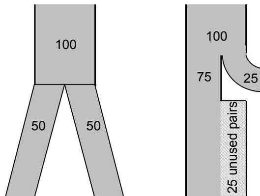
Figure 6: Examples of a join weld (left) and a drop weld (right) used for feeding a street. The figures show the number of fibre pairs involved.
