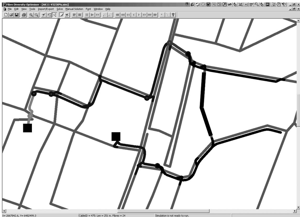
Figure 7: This figure shows the cables that are used to feed the highlighted street. The size of the cables increase as the cables get closer to the exchange. Note that the street is connected to its two feeder cables using drop welds.
