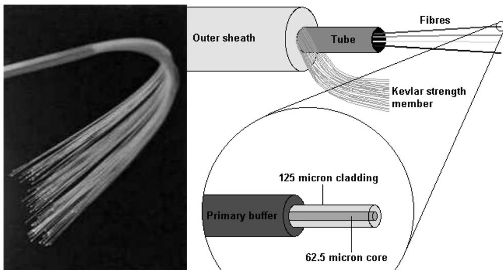
Figure 2: Fibre optic cables (left) and a schematic of their construction. Images from DataCottage.com and NewScientistJobs.com
