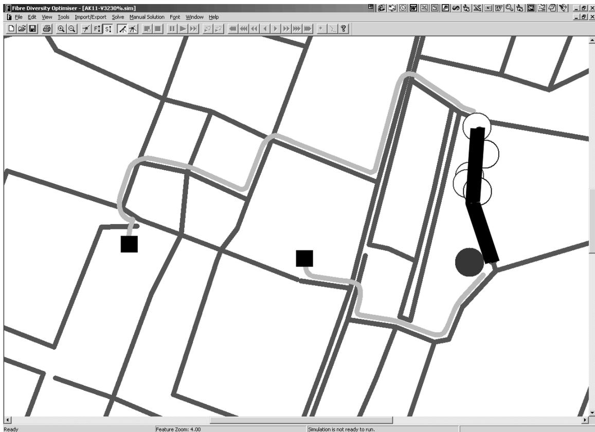
Figure 4: This figure shows the paths from a single street (highlighted) back to the exchange fibre entry points (shown by square nodes). Buildings are shown as circles, where a hollow building indicates that it does not contain a multiplexer (see below).
