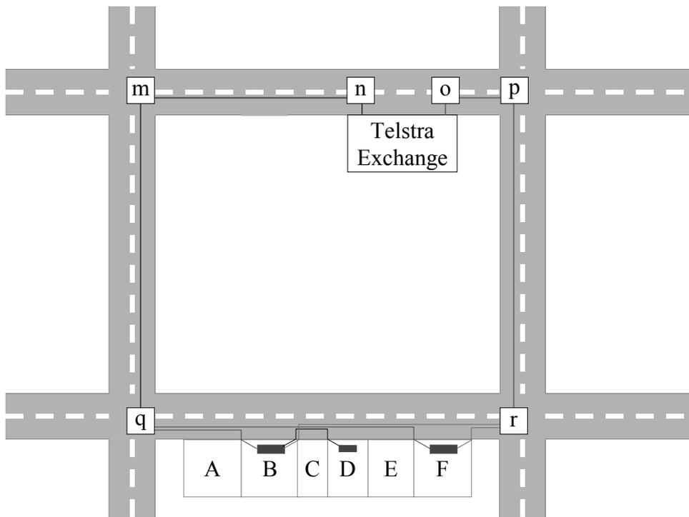
Figure 3: A sample network that feeds customer buildings B, D and F in a street. The street is connected to the exchange by two feeders, one following a feeder path from vault  $q$  through vault  $m$  to the exchange entry point  $n$ , and the other following a path from vault  $r$  through vault  $p$  to entry point  $o$ .
